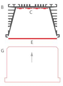
**5.** Insert the extrusion (B) together with the end cap into the mounting strip (A) and connect the power cable.
