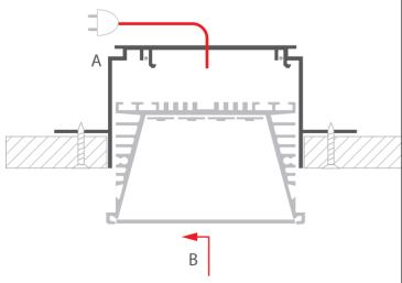
NOTE! When constructing polygonal fixtures, it is necessary to pay attention that the hooks of the assembly strip are turned to face outside the built shape. The last piece of the fixture to be mounted should be with the edges cut at an angle inwards to the inside of the polygon fixture.
