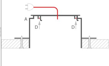
**3.** Drill holes in the extrusion (B) to run the power cable.
