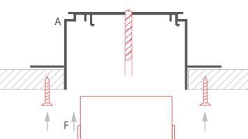
**2.** Run the power cable. Insert the mounting springs (D). The number of springs should be: 4 for 1-meter long profiles, 6 for 2-meters long profiles and 8 for 3-meters long profiles. First and last spring should be placed 10-15 cm from the end of the profile.
